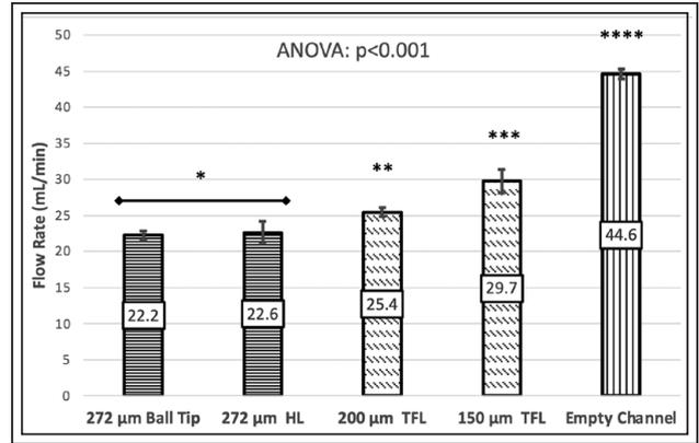
**Figure 5.** Irrigation flow rates through a flexible ureteroscope in the flexed position with various laser fibers in the working channel. Asterisks denote significant differences ( $p < 0.05$ ). Horizontal line indicates statically similar results. HL = holmium Laser; TFL = thulium fiber laser.
