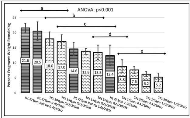
**Figure 3.** Residual fragment mean percentage using different fiber/power/frequency settings for holmium laser (HL) and thulium fiber laser (TFL). Letters **a**, **b**, **c**, **d**, and **e** represent statistically similar treatment groups.
