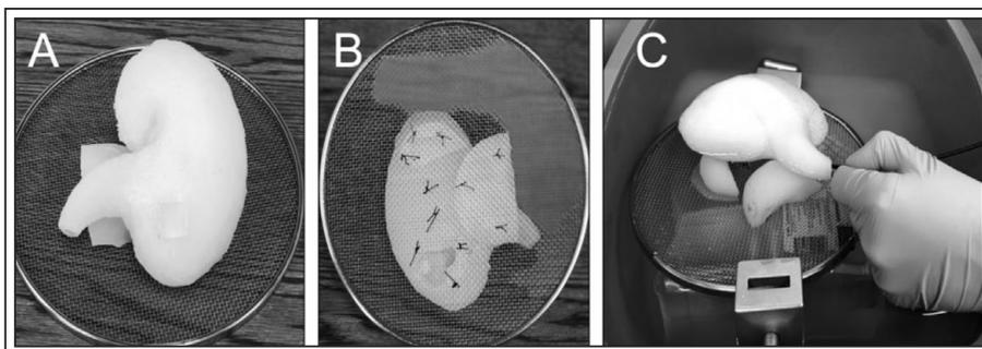
**Figure 1.** Benchtop model employed to test in situ lower pole laser lithotripsy. (A) 3D printed kidney attached to 2 x 2 mm metal mesh. (B) 1 cm BegoStone in the lower pole. (C) Ureteroscopy setup.
