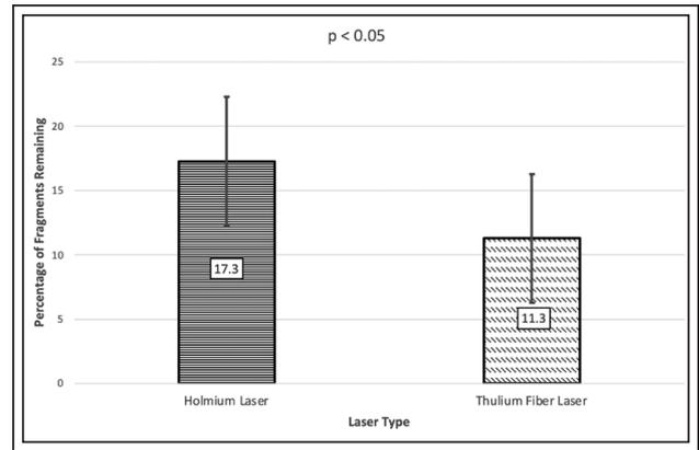
**Figure 2.** Comparison of mean percentage of remaining BegoStone fragment weight after lasering with either holmium laser or thulium fiber laser.
