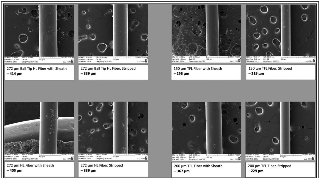
**Figure 4.** Laser fiber diameters as measured using scanning electron microscopy at 202X magnification for holmium laser (HL) fibers and thulium fiber laser (TFL) fibers.
