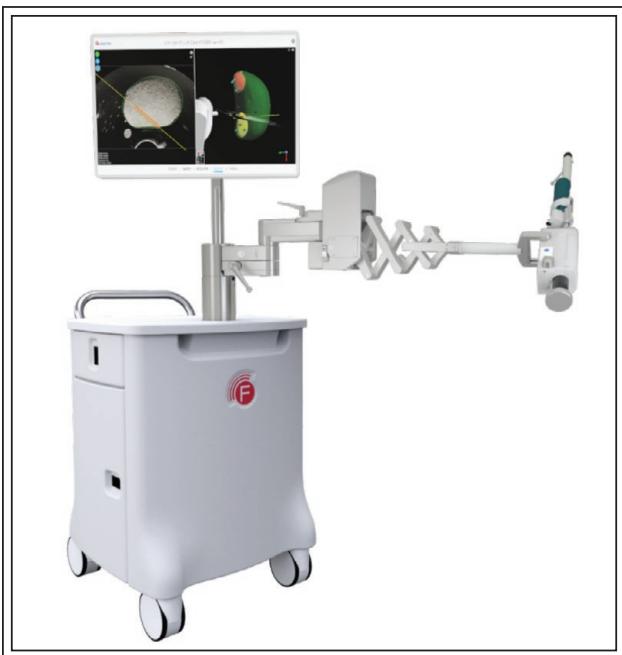
Figure 3. The TRUS probe mounted onto the Fusion Bx semi-robotic arm.
