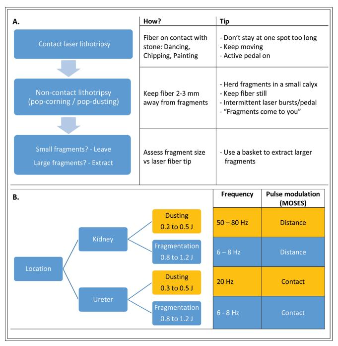
**Figure 5.** Summary of ureteroscopic laser lithotripsy treatment techniques **(A)** and settings **(B)** when using a high-power holmium laser.
